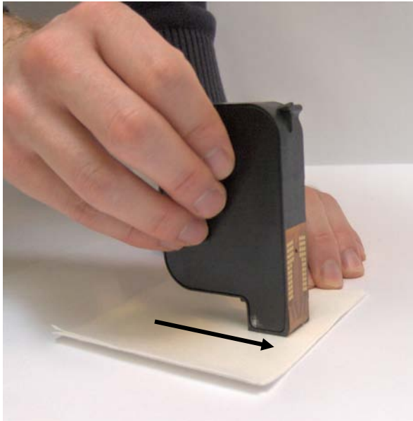
Figure 50: Cleaning the nozzle plate
